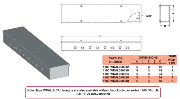
The 1100 DAL are used as junction or pull boxes and are suitable for surface mounting with a screw cover. Boxes and covers are made of high quality 12 GA aluminium. Four internal mounting holes, bonding screw and attachments are provided. Two sides have concentric knockouts (1/2" - 3/4" knockouts are standard).
